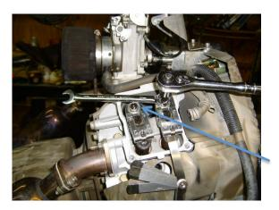
**Disconnect the battery cable and remove the spark plugs.** Set the valves on a <u>cold</u> engine, remove your valve covers (10mm wrench), spark plugs, and engage the clutch (if you are turning the prop to turn the crank). Turn the crank shaft/prop counter-clockwise until you see the valves
