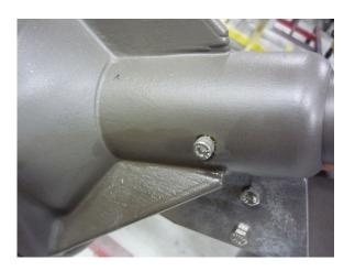
Remove the pressure release bleed screw and grease the drive. Grease until clean grease comes out the bleed screw hole. Run the engine one minute, wipe off the grease that escapes and then replace the bleed screw.
