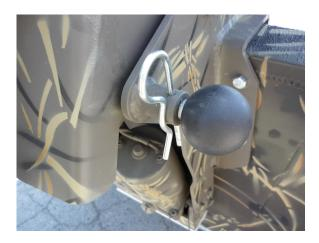
To engage, stand on the oil filter side of the engine facing the boat. While lifting the engine with your left hand, raise the engine upward to line up the tab on the base plate with the engine mount plate. Push the travel lock ball inward to lock the engine upward. Secure the travel lock with the travel lock pin.
