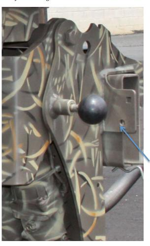
Align the motor to the center of the boat then mark the mounting holes and drill using a 3/8" drill bit.
