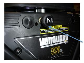
The 37EFI engine does not have a choke – it automatically richens the fuel during start up.
