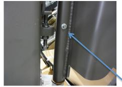
Grease the throttle cable on both ends. Also, spray a water resistant silicone spray on the throttle lever. To prevent cable freezing, remove the cable and soak in WD-40 for two hours each year.
