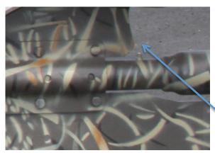
Locate the drive lubrication bleed screw located on the drive casting on the lower drive assembly.
